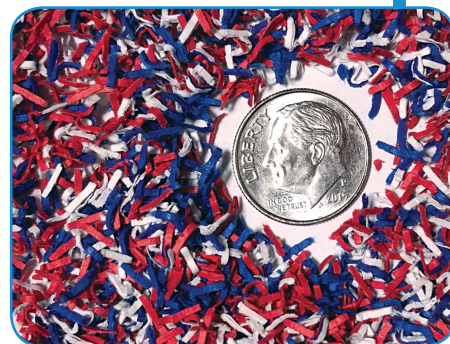
Paper media shredded particles are 0.8mm x 4.5mm in size
