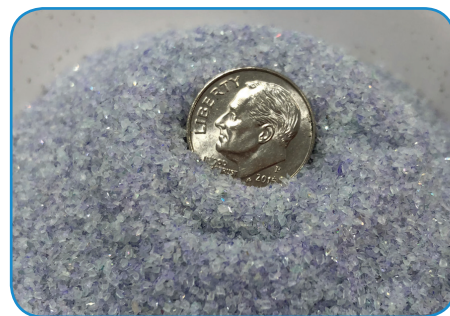
Optical media particles are <math> < 1.5\text{mm}^2 </math>, nearly as fine as salt
